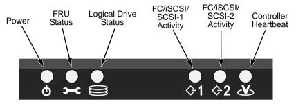
Figure 1. VTrak M500f/i/p Front Panel LEDs
